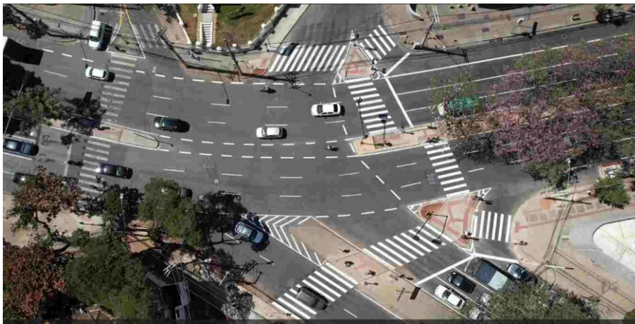
Fig. 5 Implementation of islands and new crosswalks at the intersection of Contorno Av. and Getúlio Vargas Av.
