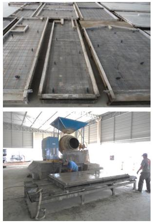
Fig. 1 Rebars positioned and panel concrete application.
