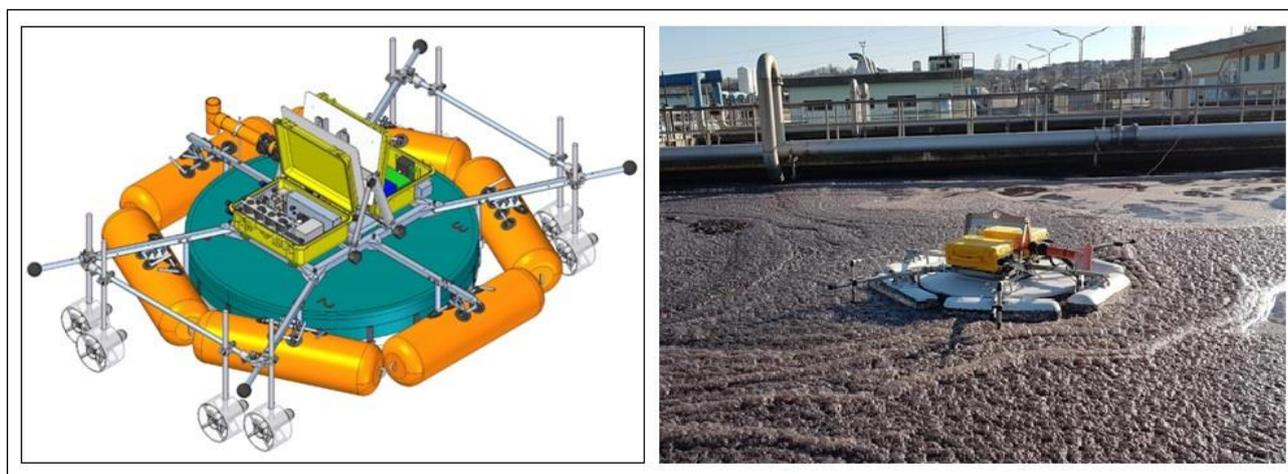
**Fig. 1** 3D view of LESSDRONE (left); LESSDRONE in the oxidation tank during a measurement (right).
