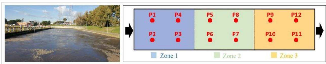
Fig. 3 East Rome WRRF oxidation tank (left); the measuring points and the three diffuser density zones in the tank (right).
