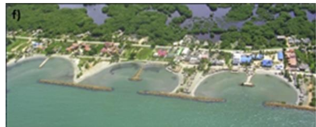
Fig. 7 Examples of detached breakwaters being used to protect beaches in tourist areas [18].
