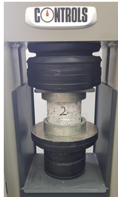
Fig. 9 Compressive strength testing of sled-hardened RCA subbase cores.
