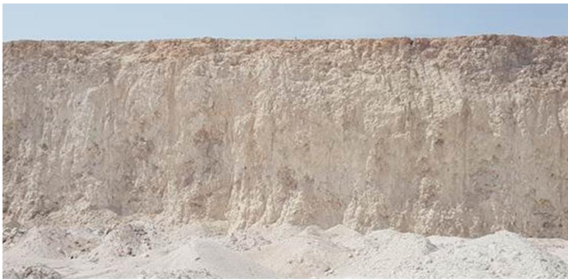
Fig. 1 Limestone quarry with disseminated clay contamination (brown colour) across the excavated face
