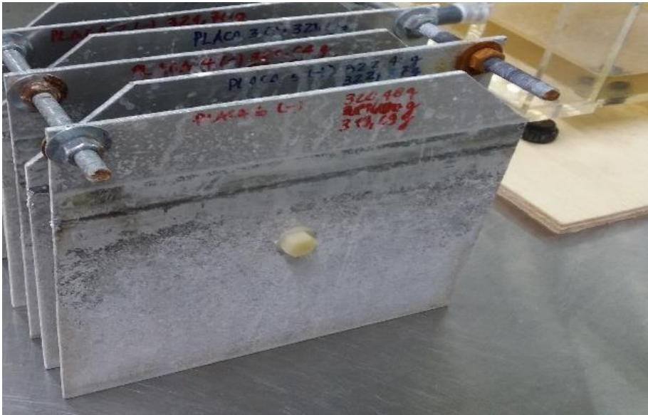
Fig. 2 Assembly of the electrode plates of the electrochemical reactor tank.
