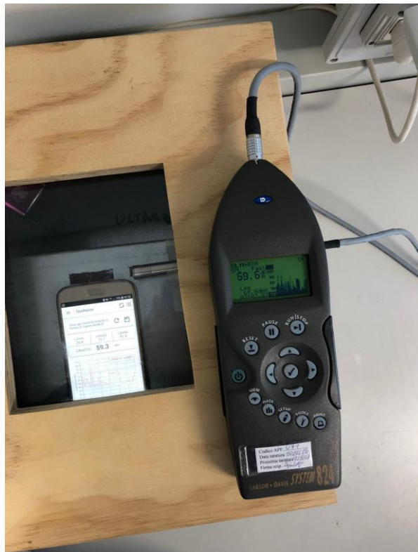
Fig. 2 Calibration of a smartphone paired to a sound-level meter: the sound level indicated by the smartphone and that displayed by the sound-level meter are compared through the control window.
