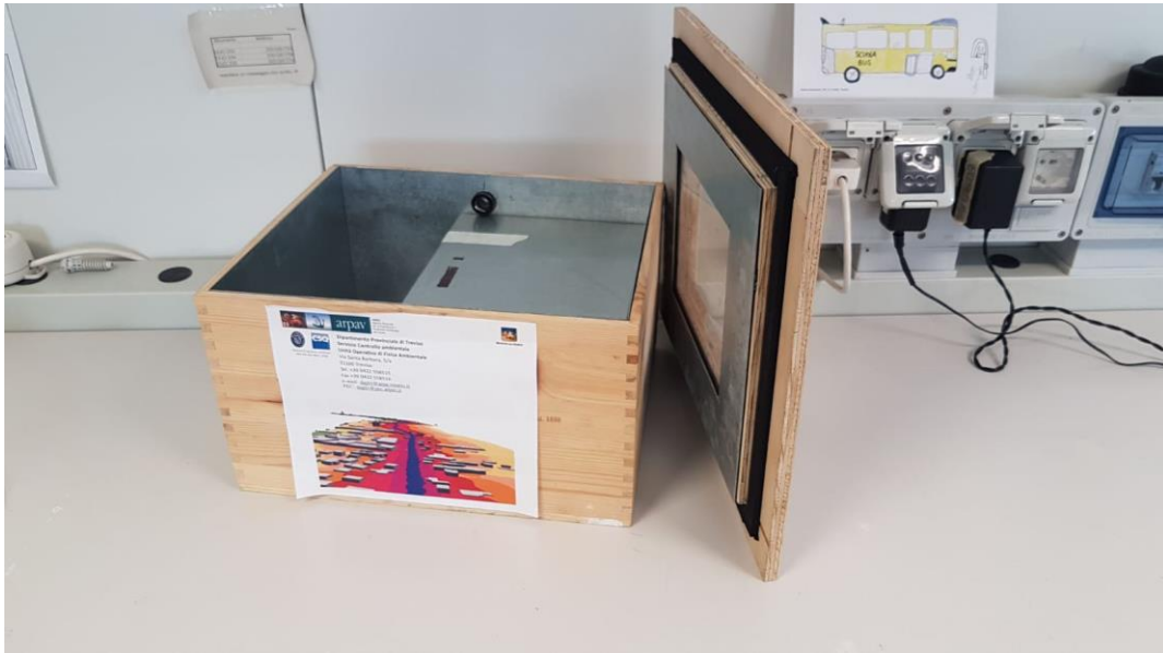
Fig. 1 Reverberation chamber for smartphones calibration; the photo shows the reverberation chamber, with the walls covered by the metal sheet; the lid with a closure seal of expanded rubber with a density of 130 \text{ kg/m}^3 ; the control window in Plexiglas.
