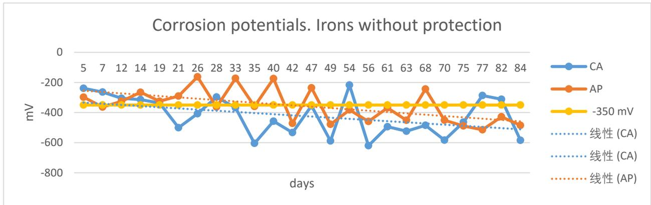
Fig. 2 Corrosion potentials. Irons without protection.
