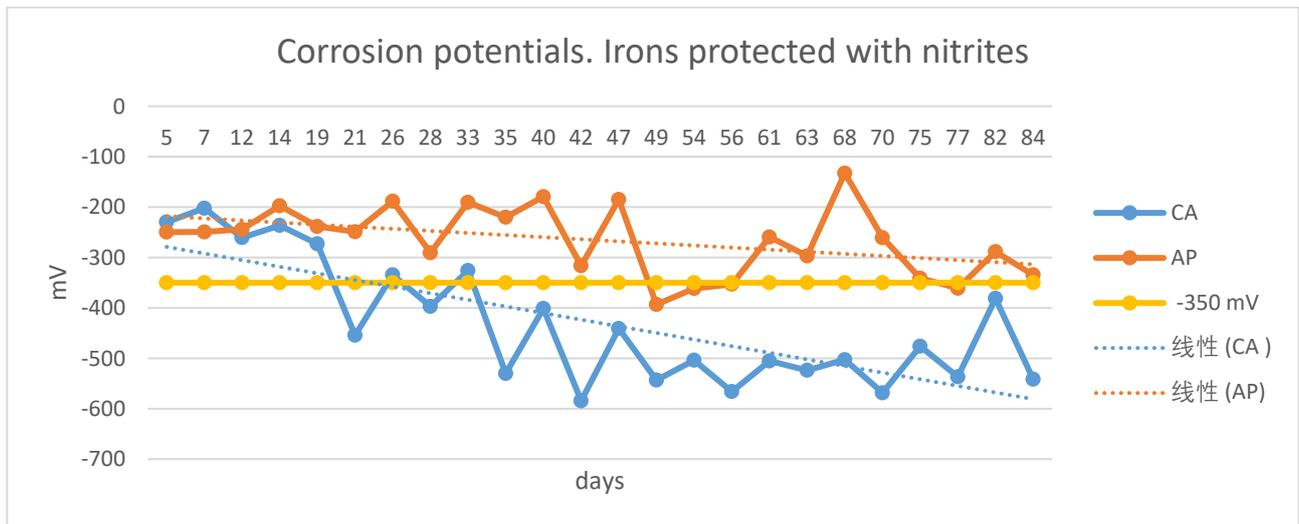
Fig. 3 Corrosion potentials. Irons painted with nitrite.
