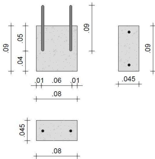
**Fig. 1 Sketches of the prismatic specimen.**
