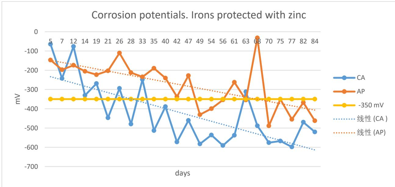
Fig. 4 Corrosion potentials. Irons painted with zinc.
