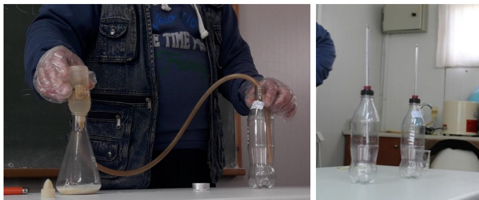
Figure 5 Left Photo: We Put Grated Marble Into the Conic Flask and Then Poured HCl Into It. The Produced \text{CO}_2 Was Collected Inside the Bottle on the Right. Right Photo: One Bottle Contained \text{CO}_2 and the Other One Atmospheric Air. We Put Thermometers Inside Both of Them.
