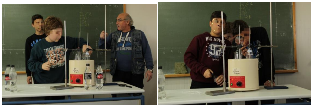
Figure 6 Left Photo: We Put the Bottles in the Beige Tank and Filled It With Water. Right Photo: As We Were Heating the Water of the Tank, So Were We Heating the Gases in the Bottles as Well, We Measured the Temperature of Each Gas Every 3 min.
