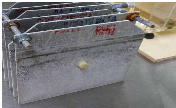
Fig. 2 Assembly of the electrode plates of the electrochemical reactor tank.
