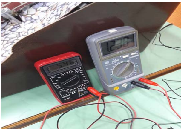
Fig. 9 Measuring voltage and current (photo authors own).
