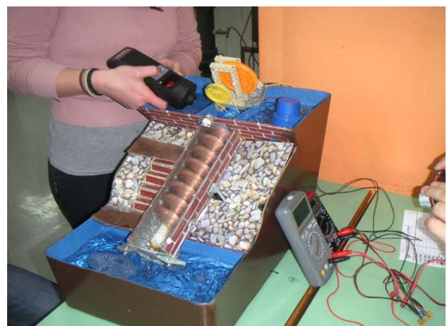
Fig. 8 Current and voltage measurements with two polymeters and rotation speed measurements with an electronic handle rotation meter (photo authors own).
