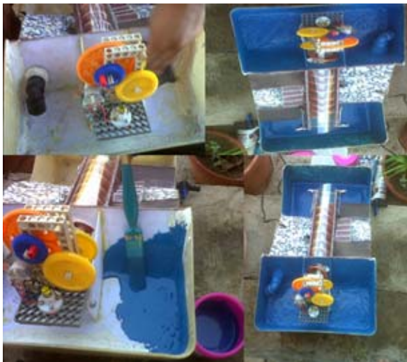
Fig. 6 Views of the whole system flume tank and details concerning its various components (photos authors own).
