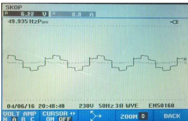
Fig. 7 Three-phase inverter output voltage when dc input voltage is 12 V and boost converter worked on 95% duty cycle (Maximum boost effect by the ANN controller).
