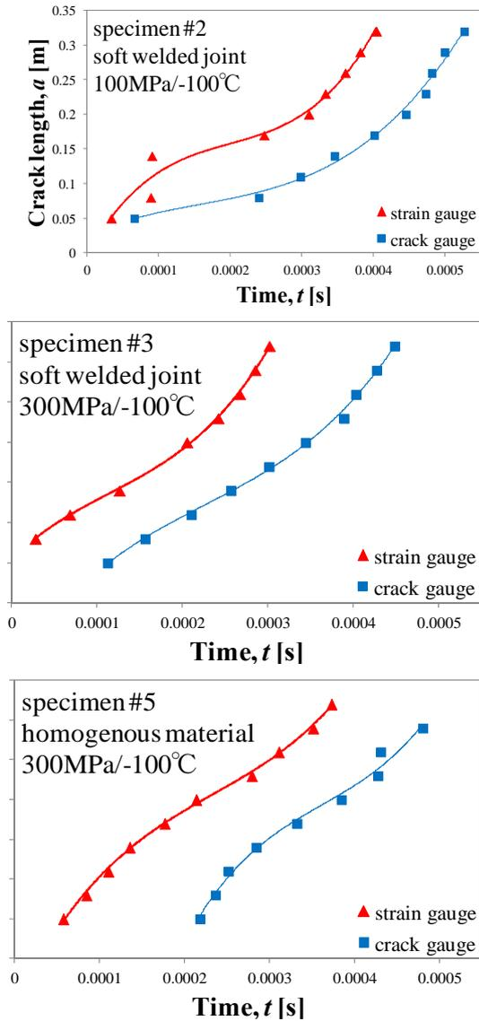
Fig. 4 Signal histories of strain gauges and crack gauges.
