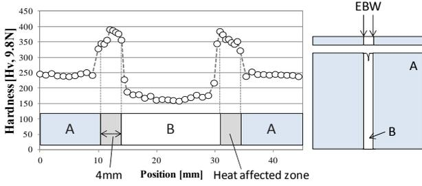
Fig. 8 Hardness distribution of soft welded joint.
