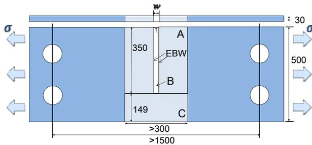
Fig. 1 Configuration of whole test specimen.
