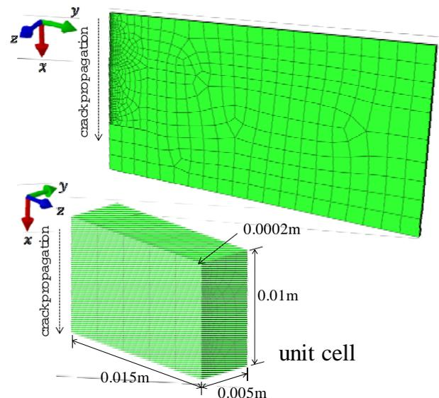
Fig. 7 Overview of the model used in FEM analysis.
