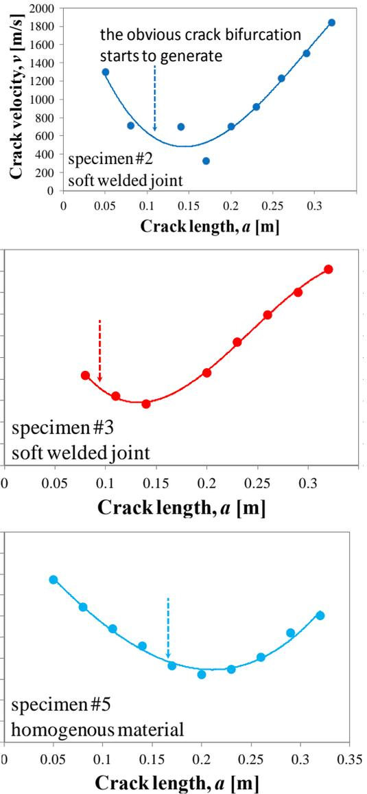
Fig. 5 Comparison of crack propagation velocity.
