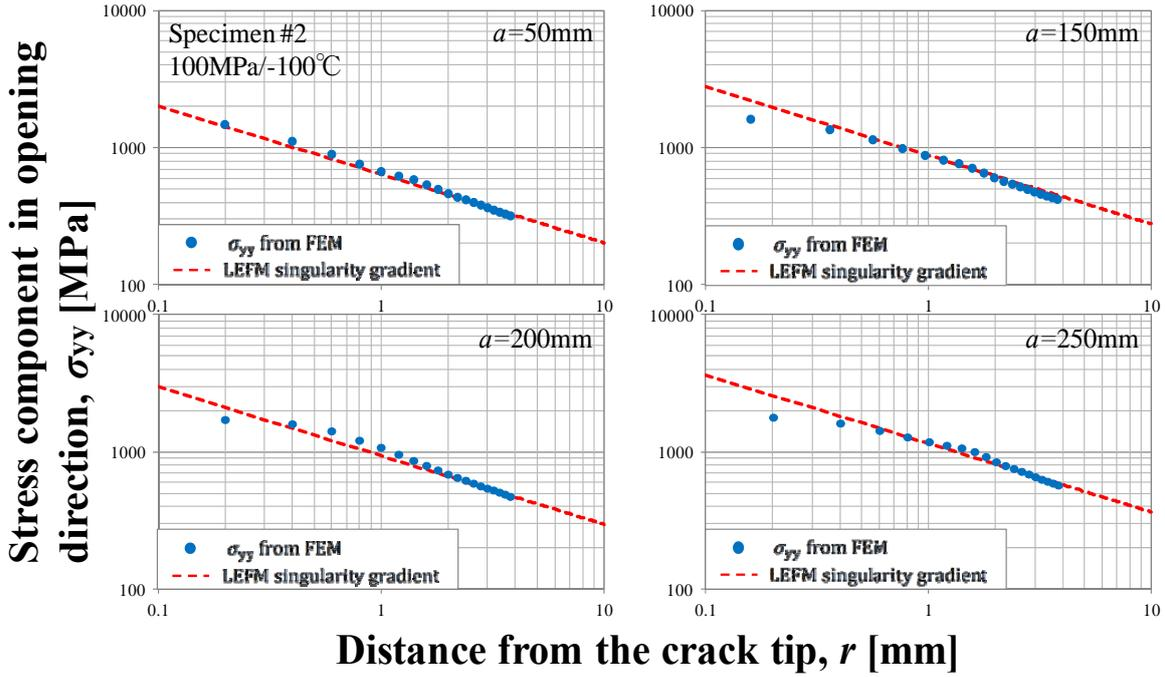
Fig. 9 Log-log plot of distance from crack tip vs. opening stresses.
