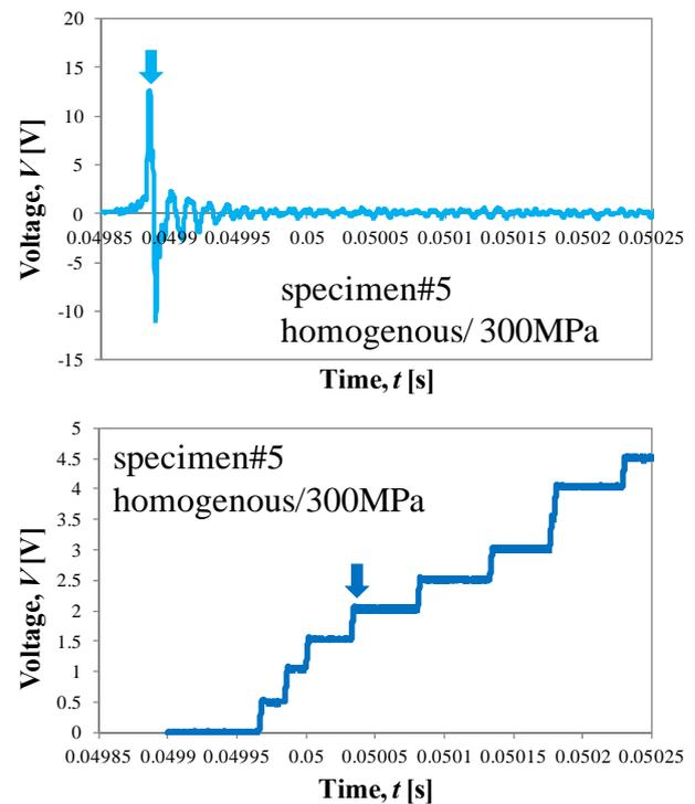
Fig. 3 An example of signals acquired by crack gauges and strain gauges at crack length of 140 mm.
