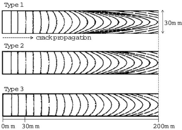
Fig. 11 Three types of curved crack tips.
