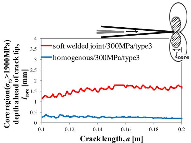
Fig. 14 Comparison of the length of high stress area.
