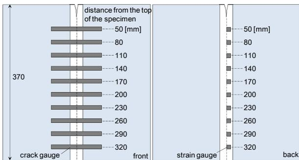
Fig. 2 Schematic illustration of the instrumentation.
