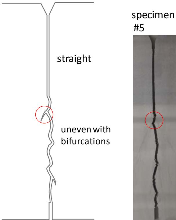
Fig. 6 Crack meandering of specimen#5.
