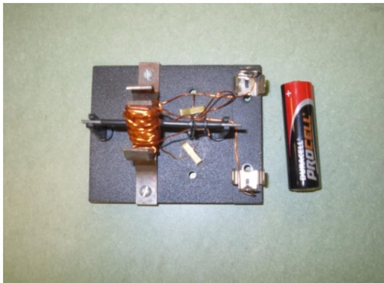
Figure 12 The Working DC Motor
