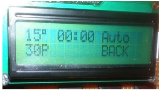
Figure 6 LCD Display When Automatic Option Been Selected
