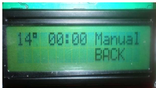
Figure 7 LCD Display When Manual Option Been Selected
