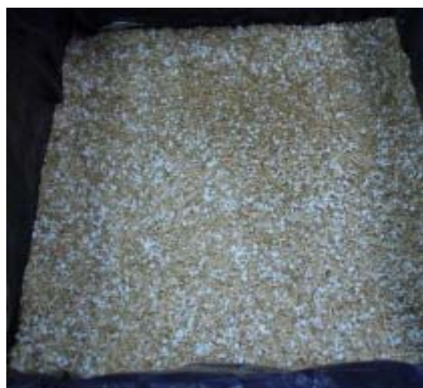
Fig. 2 Agglomerate of Wood Pellets with Polyurethane Residue
