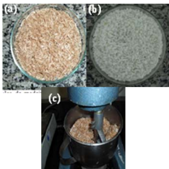
Fig. 1 (a) Wood Particles, (b) PU Solid Granules and (c) Mixture PU with Pre-Polymer and Water
