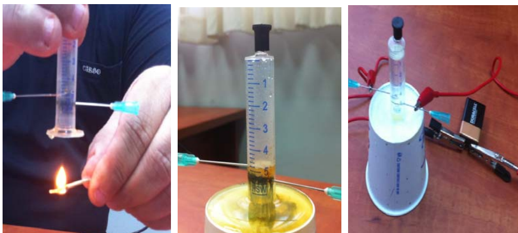
Figure 5 Plastic Syringe Apparatus for Electrolysis Designed by A Participating Teacher in the Workshop
